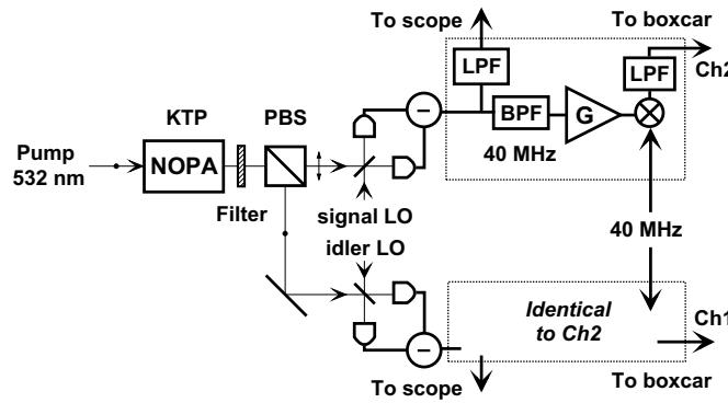
Figure 14: A schematic of the experimental setup. NOPA, non-degenerate optical parametric amplifier; LOs, local oscillators; PBS, polarizing beam splitter; LPFs, low-pass filters; BPF, band-pass filter; G, electronic amplifier. Electronics in the two channels are identical.
