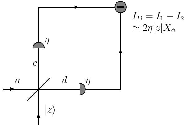
Figure 3: Homodyne detection with nonunit quantum efficiency  $\eta$ .
