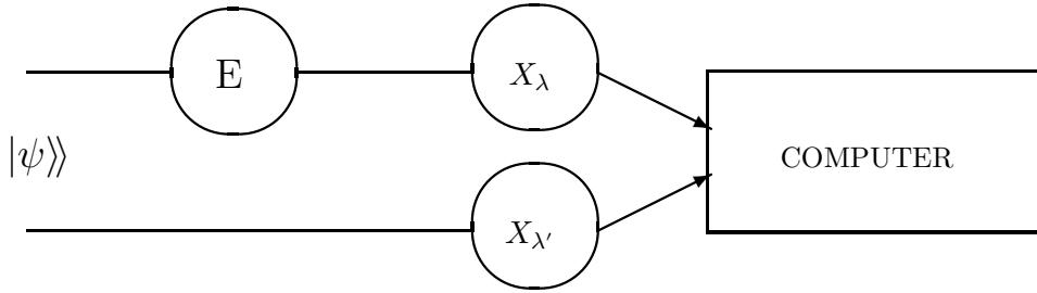
Figure 18: General experimental scheme of the method for the tomographic estimation of a quantum operation. Two identical quantum systems are prepared in an entangled state  $|\psi\rangle\langle\psi|$ . One of the two systems undergoes the quantum operation  $E$ , whereas the other is left untouched. At the output one makes a quantum tomographic estimation, photocurrent by measuring jointly two random observables from a quorum  $\{X_\lambda\}$ .
