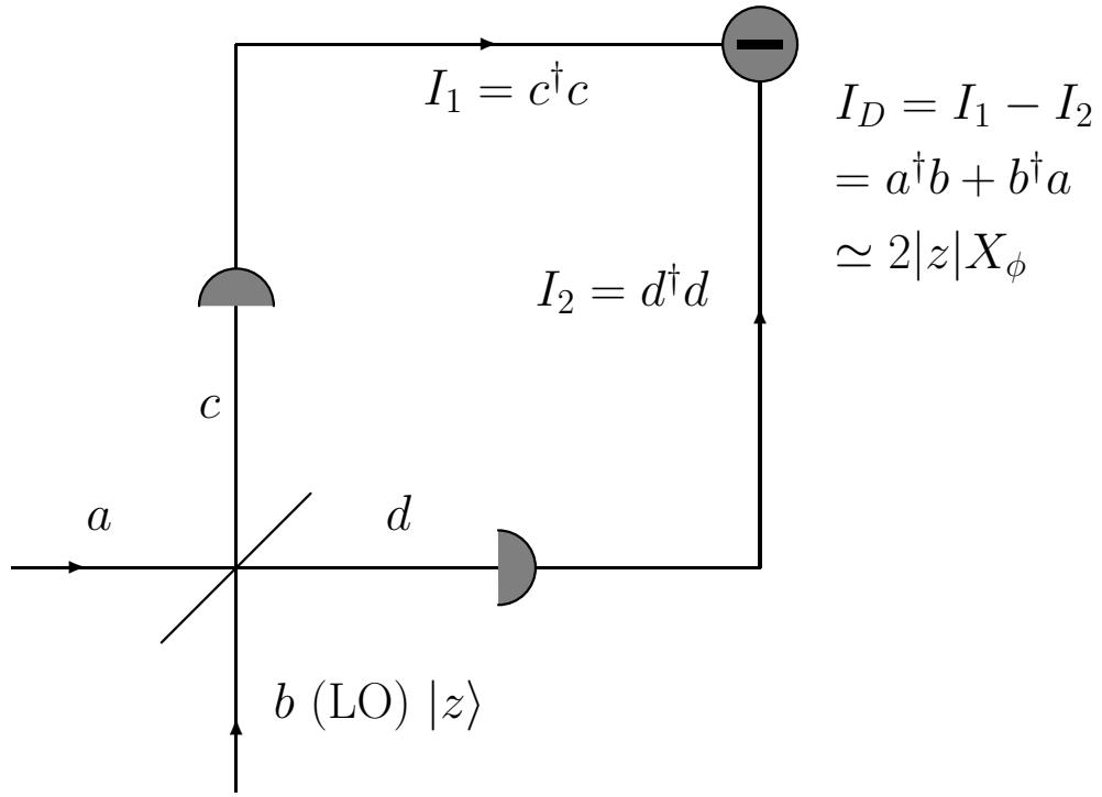
Figure 1: Scheme of homodyne detection.
