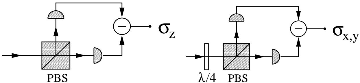
Figure 17: Pauli-matrix detectors for photon-polarization qubits.
