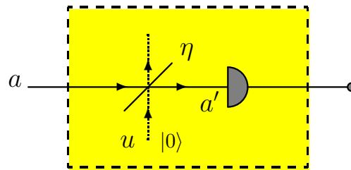
Figure 2: Equivalence of a nonideal ( $\eta < 1$ ) detector with an ideal one preceded by a beam splitter of transmissivity  $\eta$ .
